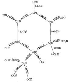
Fig. 2. Bond lengths (Å) with e.s.d.'s in parentheses; not shown on the figure: O(w)-H(w,1) 0.81 (4), O(w)-H(w,2) 0.74 (4).
