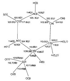
Fig. 3. Bond angles (°) with e.s.d.'s in parentheses; not shown on the figure: O(1)-S(2)-O(3) 112.5 (1), O(2)-S(2)-C(6) 104.0 (1), C(5)-C(6)-S(2) 114.4 (1), H(6)-C(6)-N(1) 110 (2), H(5,1)-C(5)-C(6) 108 (2), H(5,2)-C(5)-C(4) 110 (2), H(w,1)-O(w)-H(w,2) 101 (4).
